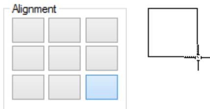
After its creation, the rectangle has 3 control points for enhanced shape control. The original corner control handle, given on creation, will control width and height of the rectangle, maintaining angle directions. The third control point will allow you to rotate and change the width and height, using the first given handle has the anchor handle.
