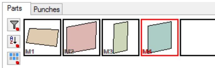
If the part changes to other slot, the name will change, in this example from M4 to M5.
