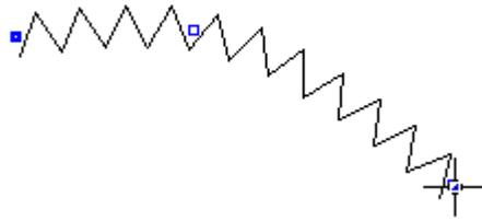
While drawing the line you can press the right mouse button and use the options to change the sawtooth line width and depth
